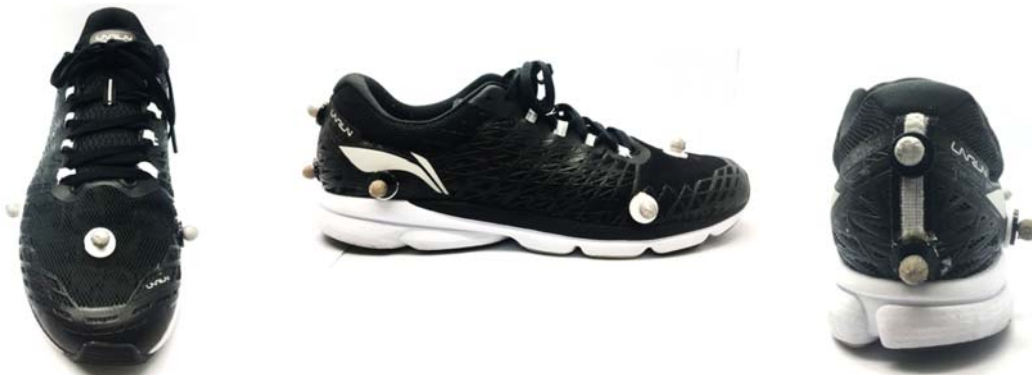
Figure 6. Marker placement in running shoes front, side and back view (from left to right).
