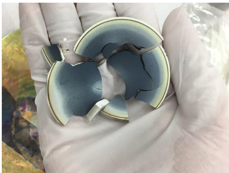
FIGURE 4.6 Broken \text{TiO}_2 target.
