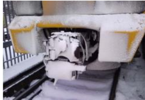
Fig 5.33 Coupler covered by snow
