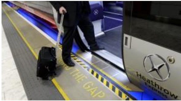
Fig 5.13 Platform gap filler
